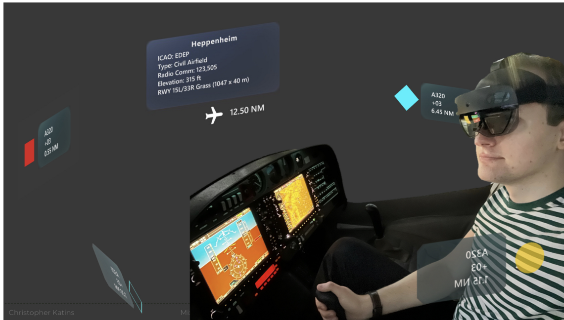
Fig. 1. In the XR application shown, Augmented Reality displays relevant information about surrounding points of interest (e.g., other traffic, airports). Pilots, for example, can benefit from these information. In this context, cognitive workload, user experience, and flight performance are augmented.
