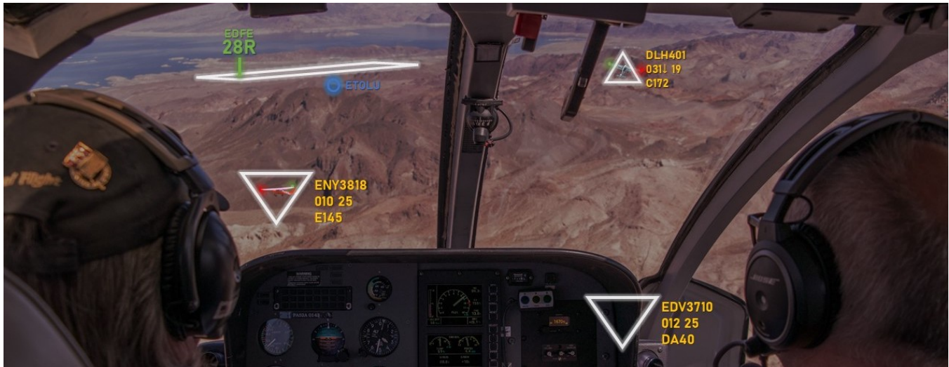
Figure 1: This mockup image shows how mixed reality could potentially be used to display relevant information about surrounding points of interest (e.g., other traffic, airports) to pilots using a head-mounted display.
